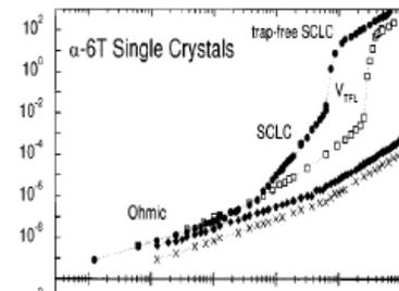
Figure 20. Current density versus voltage illustrating space-charge-limited current, from "Rodlike" Paper (I), Fig. 2.
