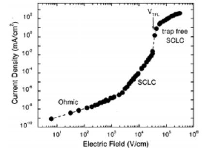
Figure 21. I-V characteristic for space-charge-limited current, from "HolePentacene" Paper (IX), Fig. 2.
