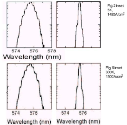
Figure 22. Emission spectrum at temperature of 5K (top) and 300K (bottom) for two injection current levels, from "Laser" Paper (XIV), Figs. 2 and 5.
